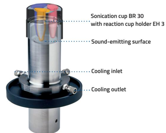
It functions like a "mini high-performance ultrasonic bath". The sample material is enclosed in a sealed vessel and is sonicated from outside via a transfer medium (e.g., iced water). The transmitted power density [W/l] is approximately 150 times higher than in a "normal" ultrasonic bath, but lower than with direct sonication with a probe.
