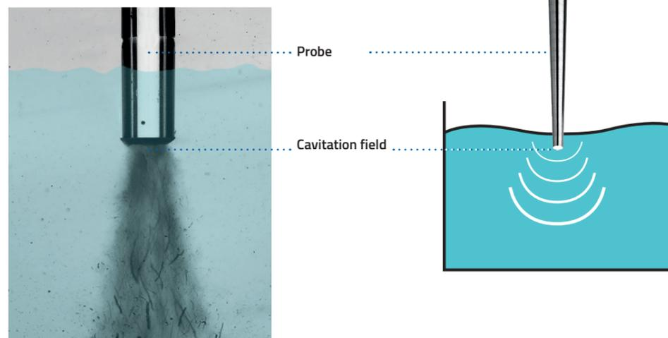
The smaller the diameter of the probe tip, the higher the power density and cavitation power for the same electrical power consumption!
