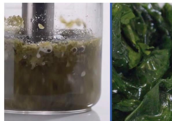
In the case of plant cells, up to 15 min are needed since the cells possess one additional shaping membrane. Thermal damage to the cell contents can be prevented by employing pulsation, i.e., periodic interruption of the power supply. In addition, respectively suitable time intervals can be set on the device. Cooling down is possible during the pulse pause.
