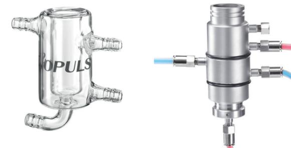
The sonicated medium is introduced from below, in other words head-on to the probe's sound-emitting surface. The sonicated medium comes into contact with the cavitation field as a result of the short distance between the sound-emitting surface and the bottom of the vessel. It has to pass through the cavitation field in order to continue flowing.
